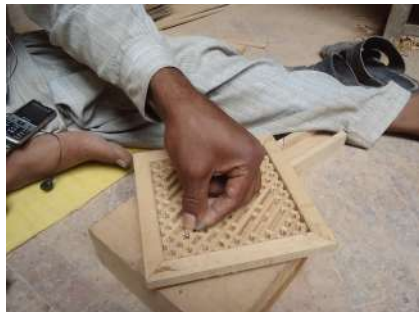
Intricate punjali being fabricated.
