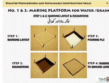
Mark layout 3'-6" x 3'-6"; dig 1'-6" after removal of 6" top soil. Place stakes on corners & pour 4" thick PLC. Raise wall in mud lime bricks.
