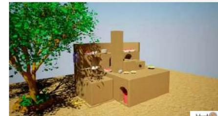
Clean burning, fuel-efficient double stove; uses small sticks or twigs. Built on raised earthen platforms, it is DRR-compliant as it can withstand rain and floods.
