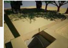
Drains will lead to a collection pit. Install an easy to remove container for collection of urine in the pit.
