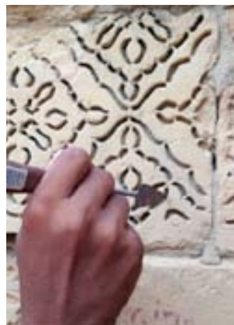
Scratching after soaking for 2 hours. Satisfactory results.
