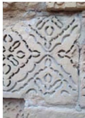
Scratching after soaking for 2 hours. Satisfactory results.
