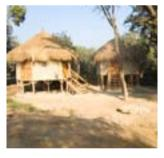
The first suite, consisting of one room and eco toilet raised on stilts in a low lying orchard areaa, was built on an experimental basis to gauge the cost of such construction. Later, 3 more were built to provide accommodation to the visitors, trainees, volunteers and personnel of the Foundation, a facility which has been used often. The construction consists of bamboo framing with dhijii cross bracing, application of lime mud plaster on matting, and a bamboo chaura thatched roof.
