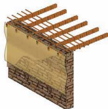
Cover walls with plastic or cloth during the curing period
