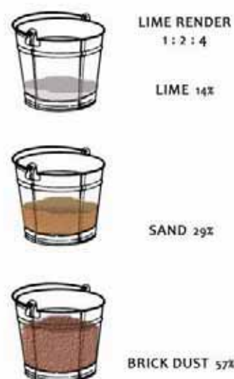
Ratio to mix Mortar for non-accessible roof
