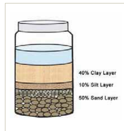
Bottle test to check clay content in soil
